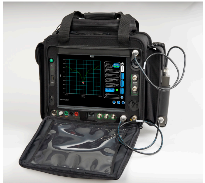
The 8800SX in Soft Case with Return Loss Bridge Connected
