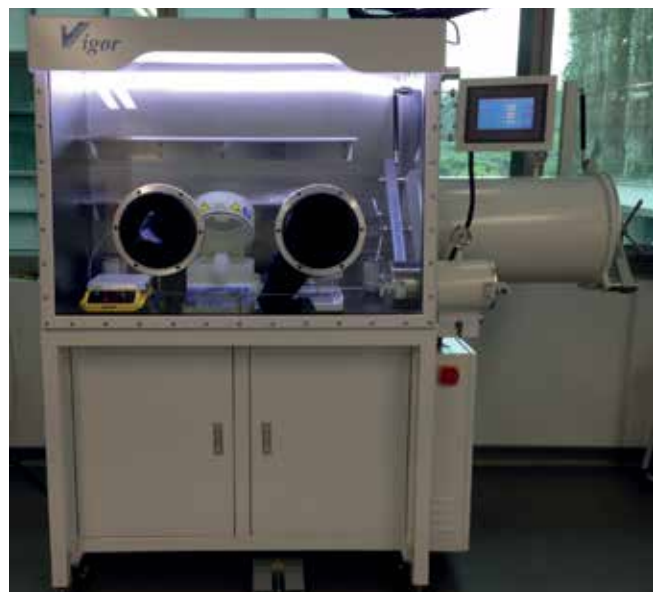
Vigor glove box with a SPIN150i table top
