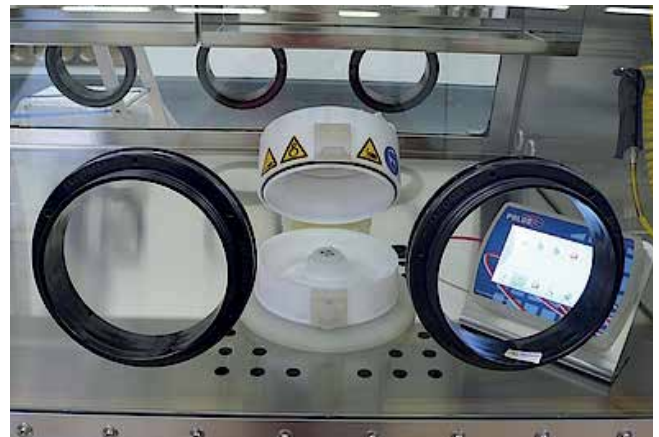
Jacomex glove box with a spincoater integration
