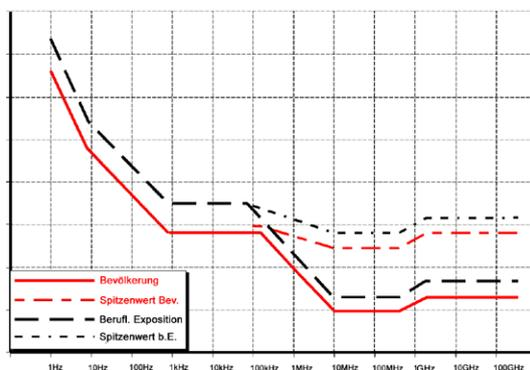
The adjacent diagram shows a visual representation of aforementioned formulas over a frequency range from 1Hz to 100GHz. The graph clearly shows that the formerly widespread broadband RF measurement instruments cannot measure and evaluate these exposure limits correctly as they are not frequency-dependent.
