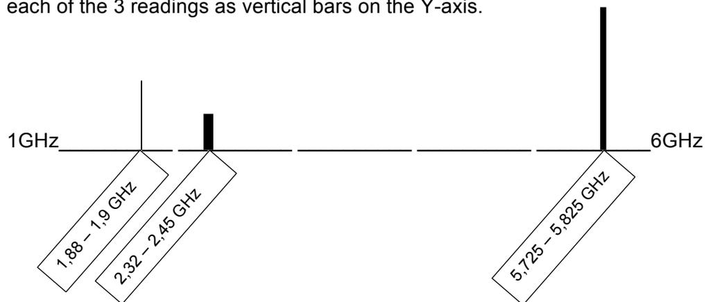
Additionally, we have also adapted the width of each vertical bar to the width of the respective frequency range of each radio application (the so-called bandwidth).
