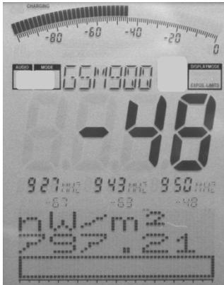
Firstly, the strongest signals are shown along with their frequencies and levels using markers, just like in spectrum mode. The large main display shows the level of the strongest signal, as usual.
