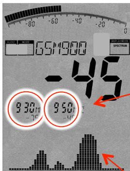
Directly beneath, a max. of 3 so-called „Markers“ are being displayed. They show the frequencies and levels of the strongest signal sources. In our example we got two Markers: Marker 1 at 930MHz at -75dBm and Marker 2 at 950MHz at -45dBm (-45dBm also is being the strongest signal and thus also shown on the main display).
