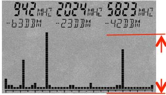
Range sets the „size“ of the visible range. Setting Range to 100dB (maximum) will give you the best possible overview of all signal sources. The vertical bars of the individual signals are virtually being “squeezed” from top to bottom to fit all signals into the display.
