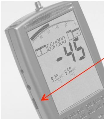
Volume can be adjusted with the volume control on the left.
