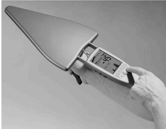
First, carefully screw the SMA adapter onto the SMA socket on the Spectran. (without much resistance). Do not use excessive force. As soon as you notice a resistance, slightly tighten the connection using the SMA-tool. Again, do not apply excessive force. Do not trigger the over torque protection. Screw by hand the SMA-adapter to the SMA socket with care (see below picture).
