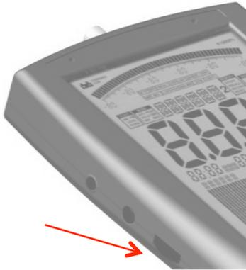
Using the Jog dial, you can activate a cursor in spectrum analysis mode. This cursor allows you to display the exact frequency and signal level of a certain point on the display.
