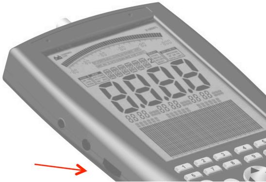
The Jog Dial replaces the up/down arrow keys (“turn” the jog dial) and the Enter key (briefly “press” the jog dial). It enables to control the complete menu navigation.
