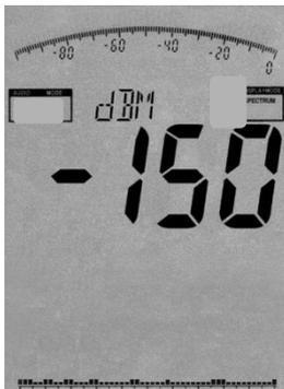
However, should the large main display show “---“, or “-150“, no signal is being received and you need to change your location or align the antenna differently. During every measurement, a little dot moves from left to right in the Graphics display. Only when this dot reaches the right border, the current measurement is finished and all readings are updated. (Depending on the settings possibly the dot is too fast for the human eye)
