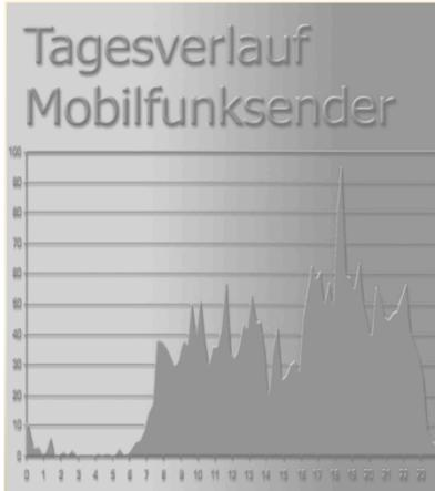
With Logger, you can start a long-term recording (Logger) in the current frequency range. Here, the highest reading and the corresponding level and frequency are regularly recorded over and over.
