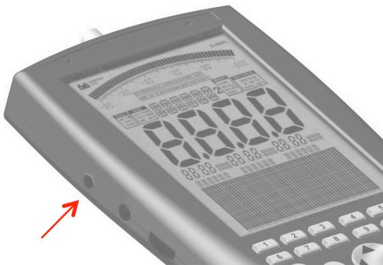
For this, connect the charger to a wall socket and plug the mini phone plug into the DC input on the Spectran. Now turn OFF your Spectran and the battery pack will be automatically charged. Full charge is reached after about 24 hours for the standard 1300mAh battery, and about 36 hours for the optional LiPo 3000mAh version.
